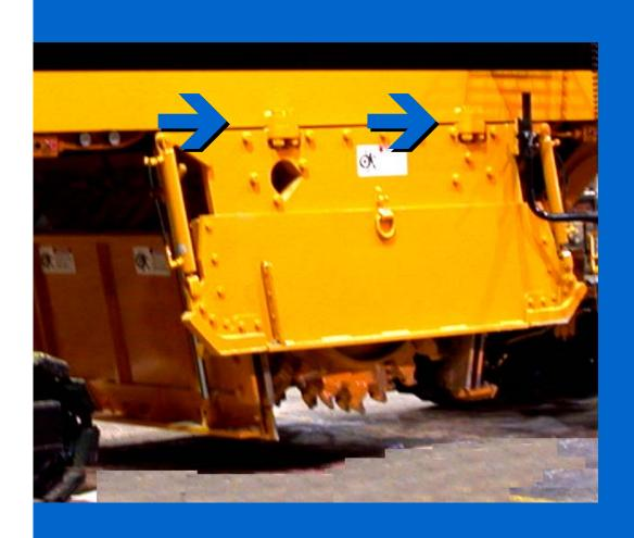
Designed for high-production and minimal downtime, all PR-600 components are modular for fast removal and maintenance. The cutter assembly bolts in place for quick changes.
