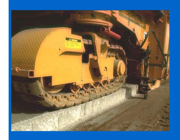
The PR-800-7 uses an improved hydraulic leg tower that lasts longer with less maintenance than earlier designs.
