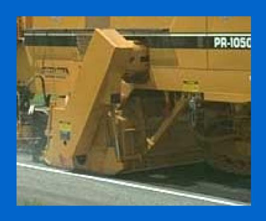
The PR-1050B comes equipped to make to 12.5 ft. wide cuts. Customers can choose bolt-on end sections to extend the cutter's capabilities even further for extra wide or heavy work on asphalt or concrete.
