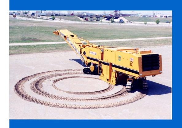
The PR-600's Fourtrack stance gives it an 8 ft. turning radius without sacrificing any of the traction needed to pull through deep, wide cuts on challenging terrain.
