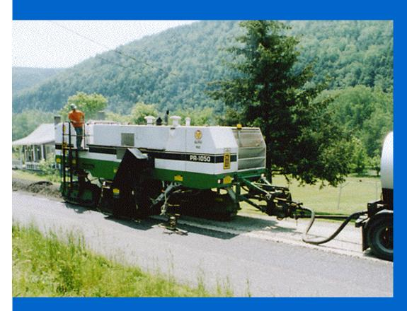
Optional bi-directional operation kit makes the PR-1050B even more productive by giving it the ability to do in-place recycling work.
