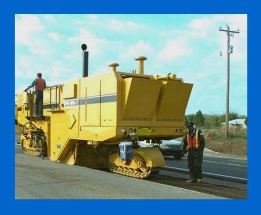
The PR-800-7 has a rugged 860 h.p. CAT diesel for high production and optimum power in tough cuts.
