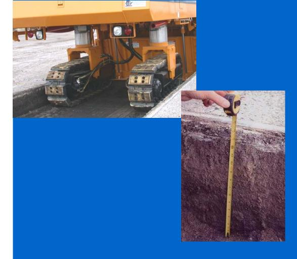
The PR-600 packs the power to make 14 in. deep plunge cuts seem like they are just all in a day's work. An operator's station ahead of cutter offers excellent visibility of the cut in urban areas and when negotiating job site obstacles.
