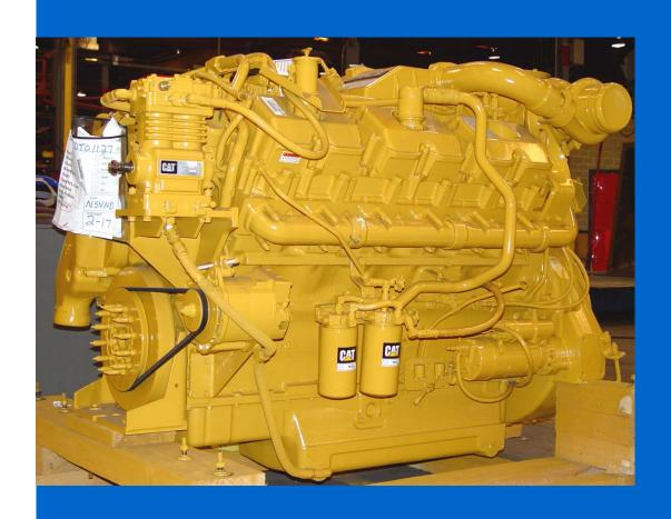
An 860 h.p. CAT diesel powers the PR-1050B's massive rotary cutter assembly. A smaller 220 h.p. CAT powers the ground drive and auxiliary systems.
