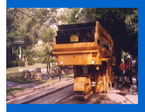
The PR-860 has a threetrack design that gives it great maneuverability and a smaller turning radius than a similar-size four-track machine. This mill is agile moving into or away from a curb line or slipping by obstacles.
