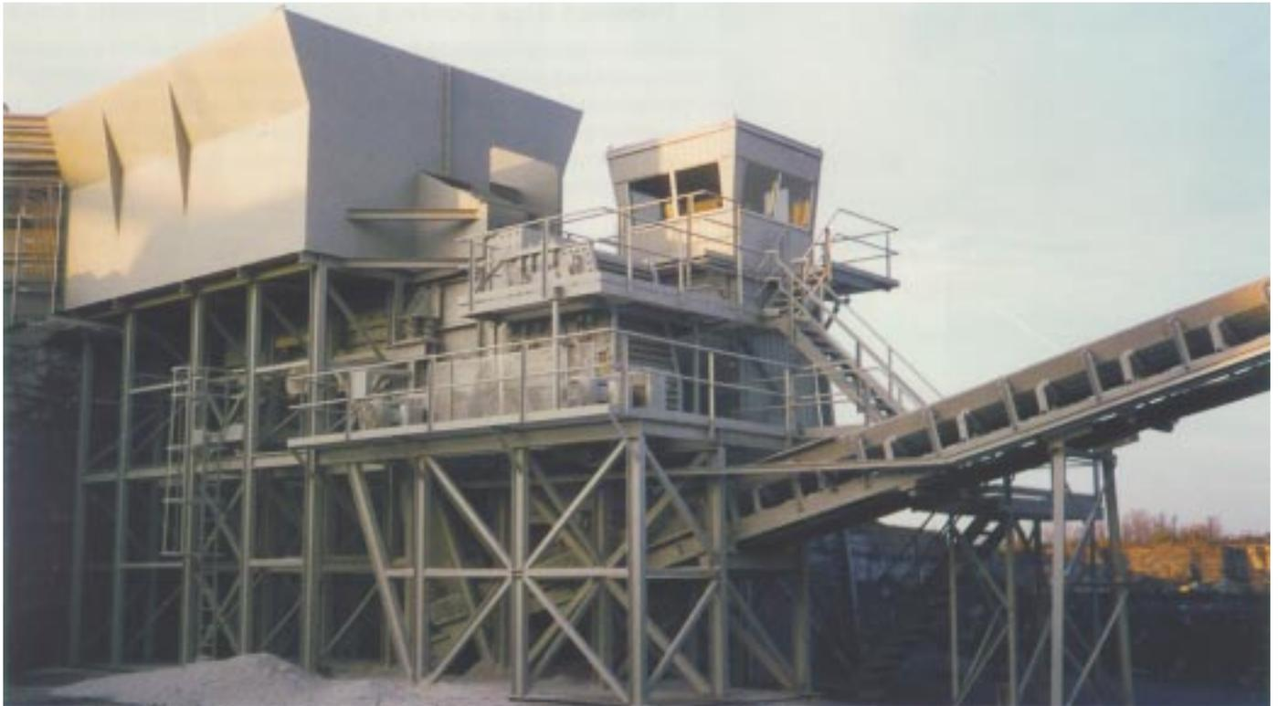
*Single impeller impact breakers can be skid-mounted or portable. Skid units, which can include feeder, grizzly and drive, are completely engineered and ready to install on piers. Portable units have the same components and a discharge conveyor on a single chassis for easy transport. Electric motor or combustion engine provide power.*
