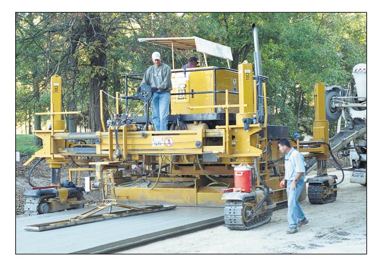
The CMI Terex SF-2204 HVW is the utility sized machine in the world's only family of Hydraulic Variable Width Concrete Slipform Pavers.
