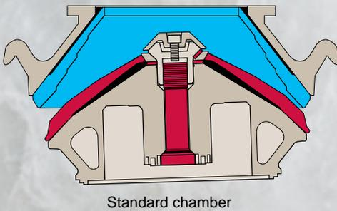
Changing crushing chambers only requires installing manganese bowl and mantle.
