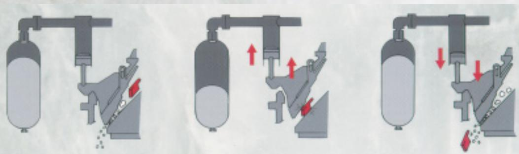
The relief system operates by forcing the bonnet upward against the system's oil pressure in the relief cylinders as an uncrushable object enters the cone's crushing chamber. The oil pressure in turn compresses a nitrogen gas bladder in the accumulator. Once the crushing cavity is cleared, the gas forces the oil back into the relief cylinder and the bonnet lowers to its original position.
